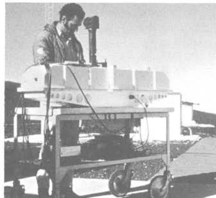
Bernard Mendonca measuring ozone with a Dobson spectrophotometer, March 1972.
