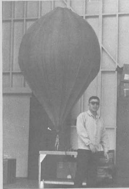
John Chin with ozonesonde at the National Weather Service airport station, Hilo, in March 1970. The MLO balloon-supported instrument used the standard Weather Bureau radiosonde transmitter and receiver at the airport.
