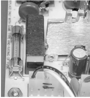
Ohmmeter to confirm that the Switch is functional, and check the two fuses next to the power supply cover as indicated in the photograph. If a fuse needs changing, ensure that AC power is disconnected, and replace the fuse with the appropriate spare.
