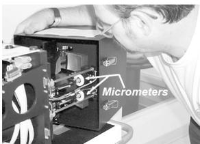
If the lamp is working fine, and light can be seen in the Viewing Ports, then the position of the micrometer should be checked. Remove the "Spectrometer" cover and check to see that the micrometer is in the correct position as indicated in the Final Test Record, and on the Log Sheet taped to the Spectrometer cover. If the Micrometer is not where the Log Sheet indicates, it should be adjusted manually and an HG test attempted again.
