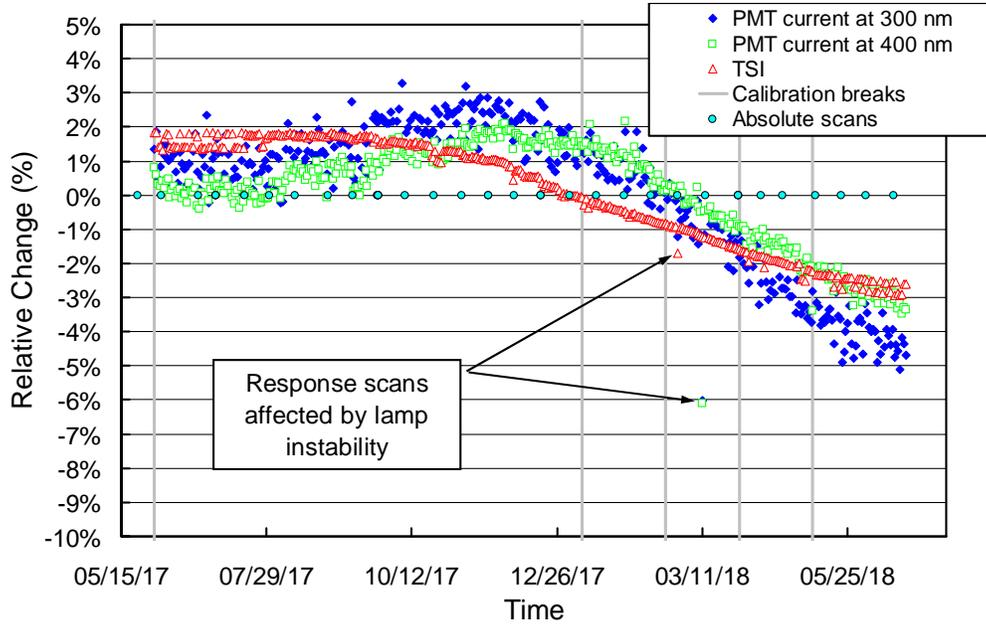
**Figure 2.** Time-series of PMT current at 300 and 400 nm, and TSI signal. All data were extracted from measurements of the internal irradiance standard and are normalized to their average. Calibration break points (Table 1) and times of absolute scans are also indicated. Arrows point to data points that were affected by the instability of the internal lamp.
