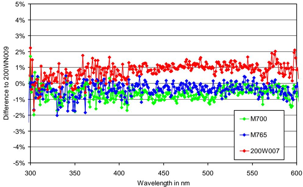
**Figure 1.** Comparison of the calibration of on-site standards M700, 200W007, and M765 with long-term standard 200WN009 on 9/24/2017.
