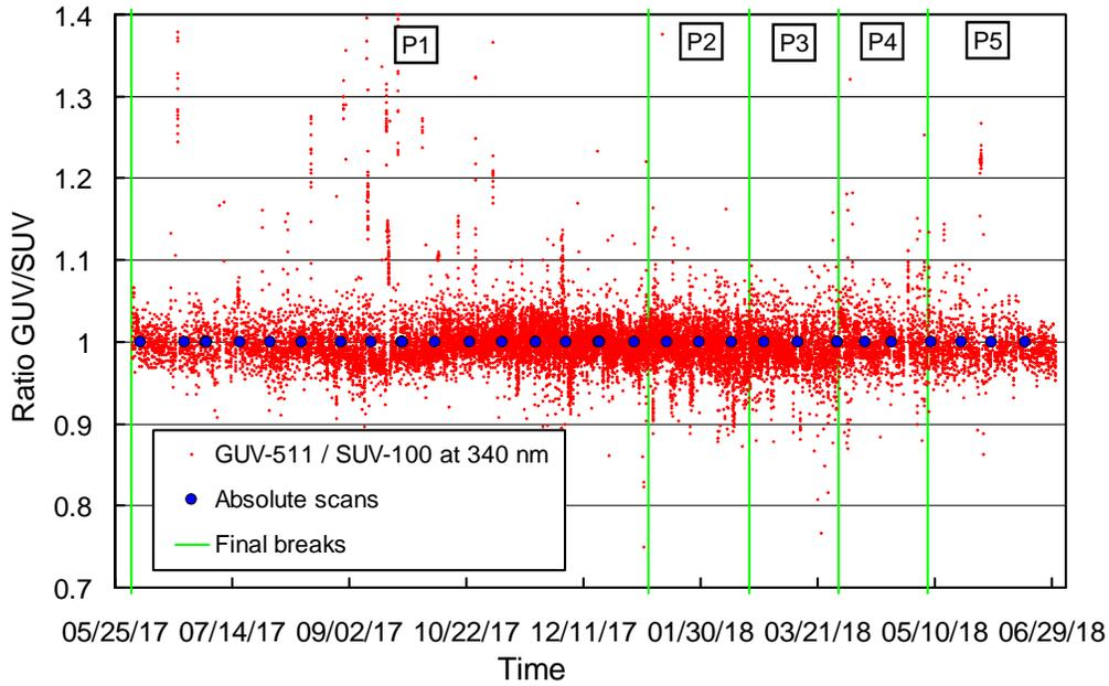
**Figure 4.** Ratio of GUV-511 measurements at 340 nm with final SUV-100 measurements. The latter were weighted with the spectral response function of the GUV-511 340 nm channel. Narrow clusters of vertical data points are caused by snow covering the SUV-100 collector.
