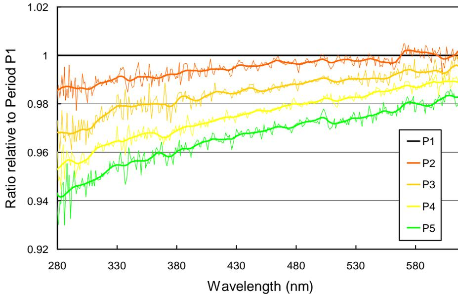
**Figure 3.** Ratios of spectral irradiance assigned to the internal reference lamp for periods P1 – P5 relative to Period P1. Heavy lines indicate smoothed ratios.
