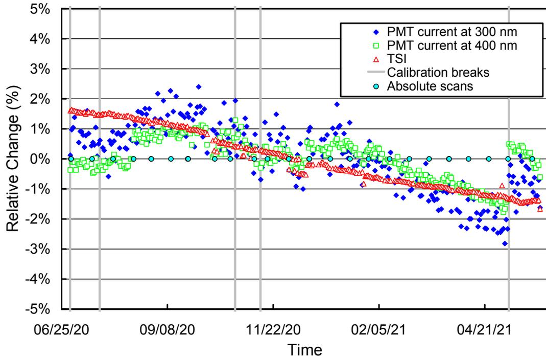
**Figure 2.** Time-series of PMT current at 300 and 400 nm, and TSI signal. All data were extracted from measurements of the internal irradiance standard and are normalized to their average. Calibration break points (Table 1) and times of absolute scans are also indicated.
