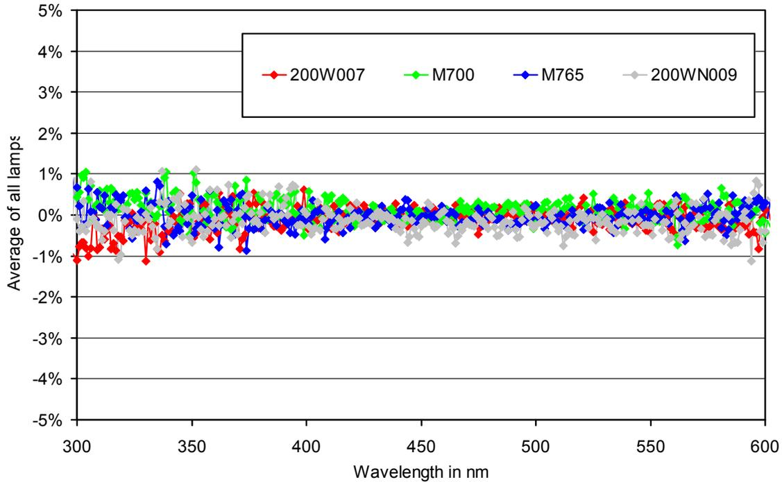
**Figure 1.** Comparison of the calibration of on-site standards 200W007, M700, and M765 with long-term standard 200WN009 on 9/22/2020.
