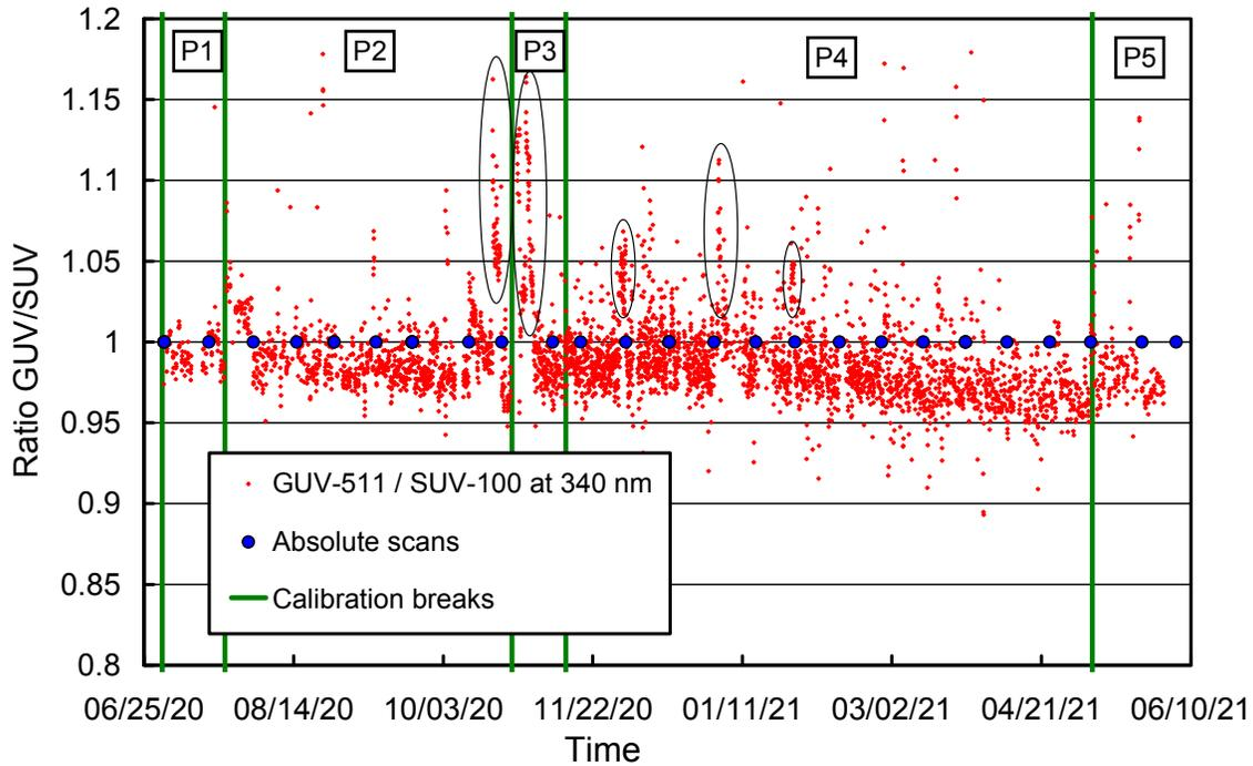
**Figure 4.** Ratio of GUV-511 measurements at 340 nm with SUV-100 measurements. The latter were weighted with the spectral response function of the GUV-511's 340 nm channel. Narrow clusters of vertical data points marked by ellipses are likely caused by snow covering the SUV-100 collector.
