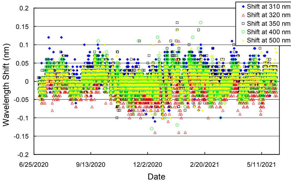
Figure 6. Wavelength accuracy check of the final Version 0 data at five wavelengths by means of Fraunhofer-line correlation. Measurements were evaluated in four-hour increments.
