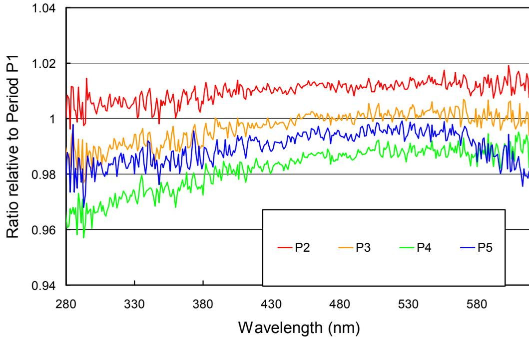
**Figure 3.** Ratios of spectral irradiance assigned to the internal reference lamp for periods P1 – P7, relative to Period P1.
