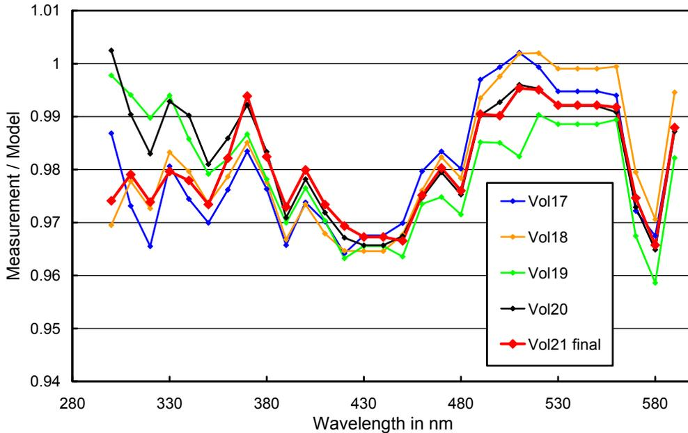
**Figure 3.** Median measurement/model ratios calculated from clear-sky solar measurements for data of Volumes 17 – 21. Ratios were averaged over 10 nm intervals (305-315, 315-325, ... 585-595 nm) before the median was calculated. There is a systematic bias between measurement and model, however, this bias is generally to within  $\pm 1\%$  for the five volumes, confirming that the irradiance scale used for processing of Volume 21 data is consistent with that used for earlier volumes.
