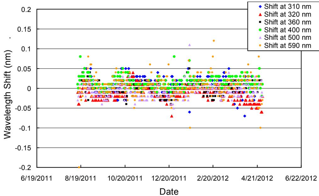
**Figure 9.** Check of the wavelength accuracy of final Version 0 data at six wavelengths by means of Fraunhofer-line correlation. The plot is based on daily measurements at noon.
