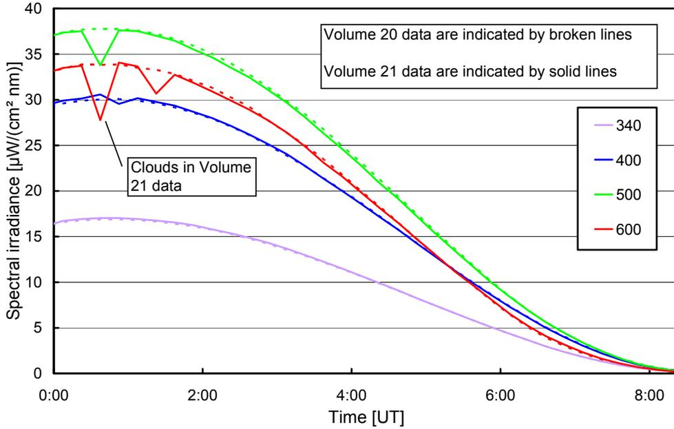
**Figure 4.** Spectral irradiance at 340, 400, 500 and 600 nm on 9/30/10 (Volume 20 data, broken lines) and 9/30/11 (Volume 21 data, solid lines). The surface albedo was 0.85 on both days. The graph indicates that measurements at the same time, one year apart, are consistent to within  $\pm 1.5\%$ .
