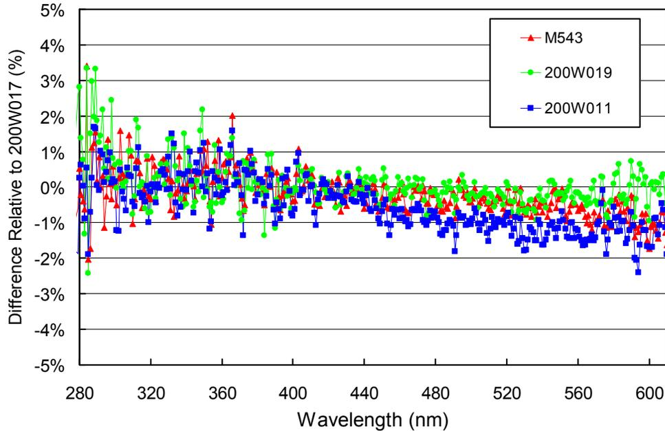
**Figure 1.** Comparison of on-site lamps M-543, 200W019 and 200W011 with the BSI traveling standard 200W017 on 02/02/2011.
