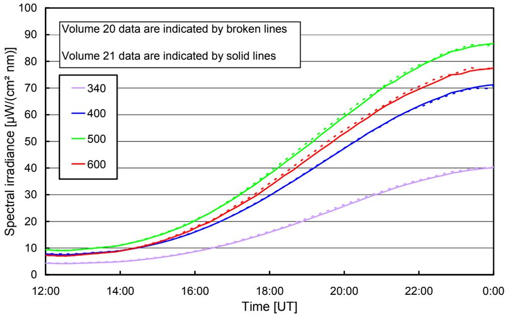
**Figure 5.** Spectral irradiance at 340, 400, 500 and 600 nm on 11/9/10 (Volume 20 data, broken lines) and 11/9/11 (Volume 21 data, solid lines). The surface albedo was 0.80 on both days. The graph indicates that measurements at the same time, one year apart are consistent to within  $\pm 1.5\%$ .
