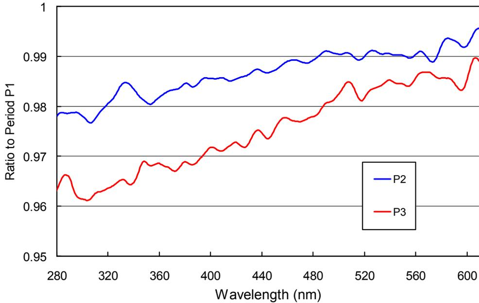
**Figure 7.** Ratios of irradiance assigned to the internal reference lamp during periods P2 and P3, relative to Period P1. Changes from period to period are smaller than 2%.
