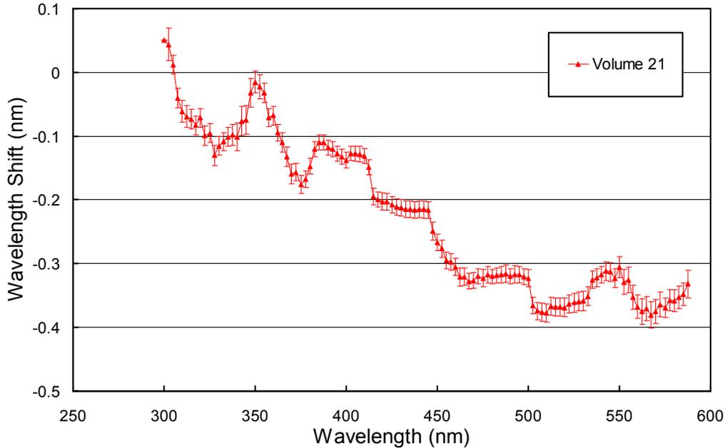
**Figure 8.** Monochromator non-linearity correction functions for the Volume 21 period. Error bars indicate the  $1\sigma$ -variation.
