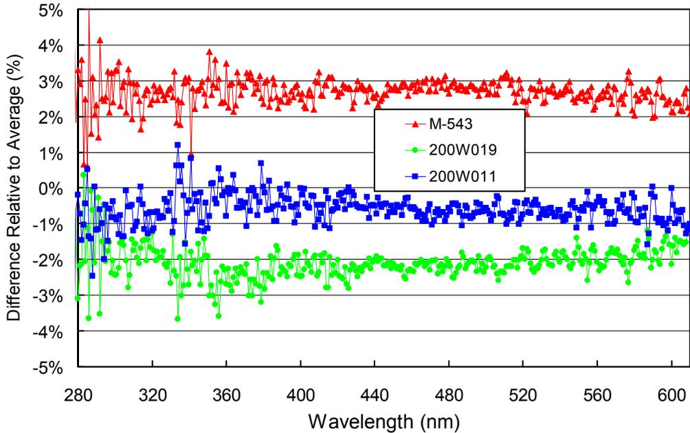
**Figure 2.** Comparison of lamps M-543, 200W019 and 200W011 with their average on 5/23/2012.
