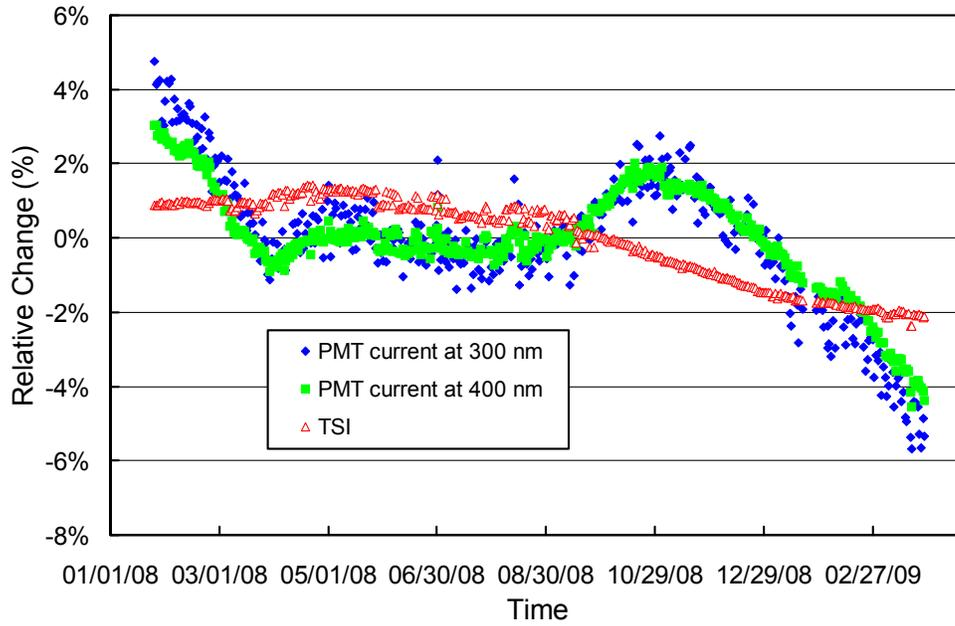
**Figure 5.3.3.** Time-series of PMT current at 300 and 400 nm, and TSI signal for measurements of the internal irradiance standard performed during the South Pole 2008/09 season. Data are normalized to the average of the whole period.
