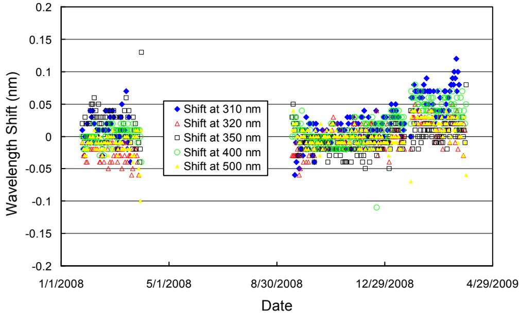
**Figure 5.3.9.** Wavelength accuracy check of final data at four wavelengths by means of Fraunhofer-line correlation. Measurement performed at 00:00 UT were evaluated for each day of the season. No data exist during Polar Night.
