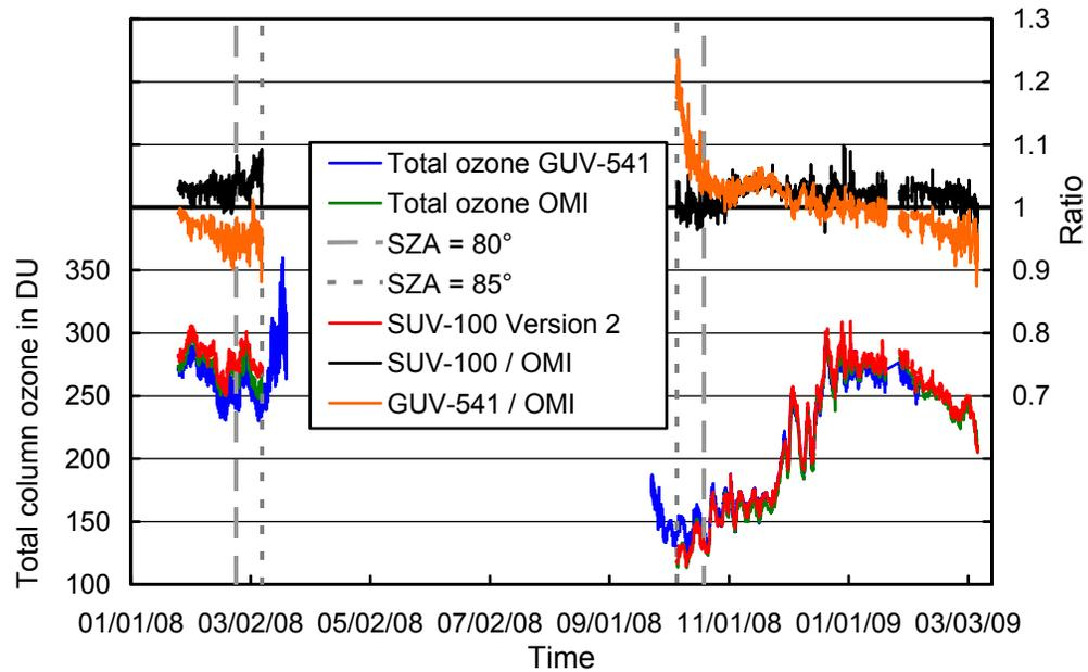
**Figure 5.3.11.** Comparison of total column ozone measurements from GUV-541, SUV-100 (Version 2 data), and OMI. GUV-541 and SUV-100 measurements are plotted in 15 minute intervals. For calculating ratios of data sets, only GUV-541 and SUV-100 measurements concurrent with OMI overpass data were evaluated.
