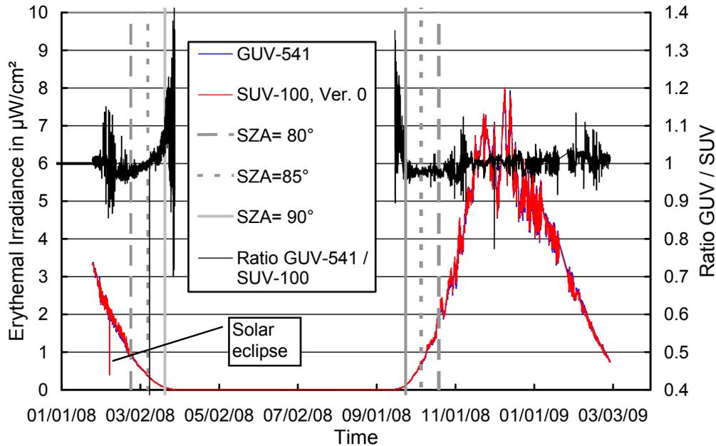
**Figure 5.3.10.** Comparison of erythemal irradiance measured by the SUV-100 spectroradiometer and the GUV-541 radiometer. SUV-100 measurements are based on “Version 0” (cosine-error uncorrected) data.
