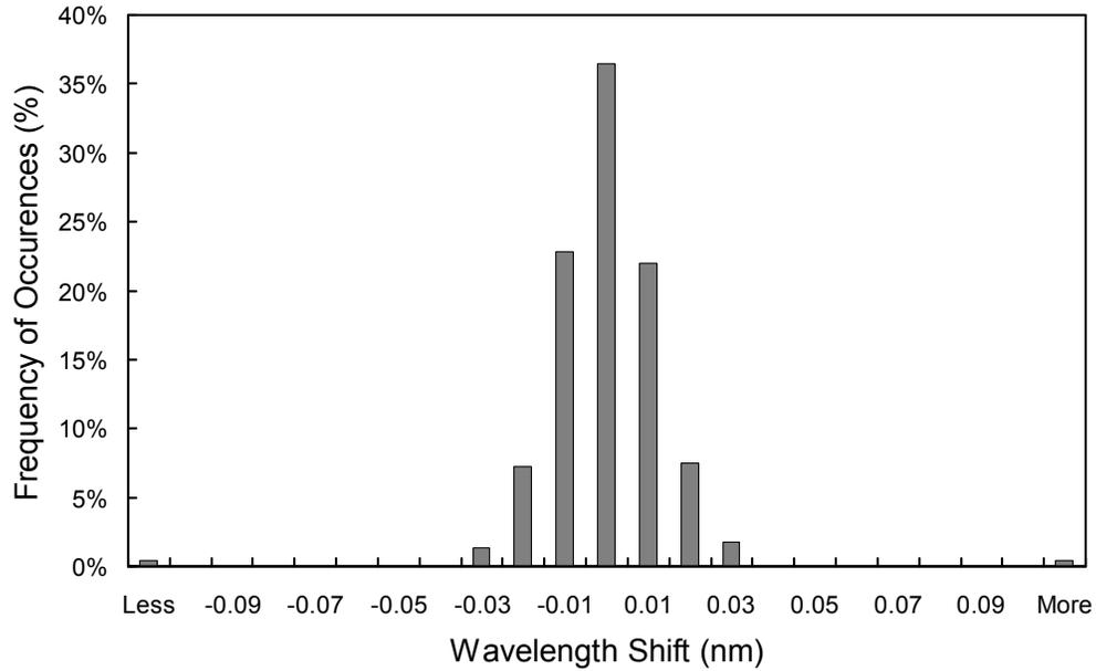
**Figure 5.3.7.** Frequency distribution of the difference of the measured position of the 296.73 nm mercury line between consecutive wavelength scans. The x-labels give the center wavelength shift for each column. The 0-nm histogram column covers the range -0.005 to +0.005 nm. “Less” means shifts beyond -0.105 nm; “more” means shifts beyond +0.105 nm.
