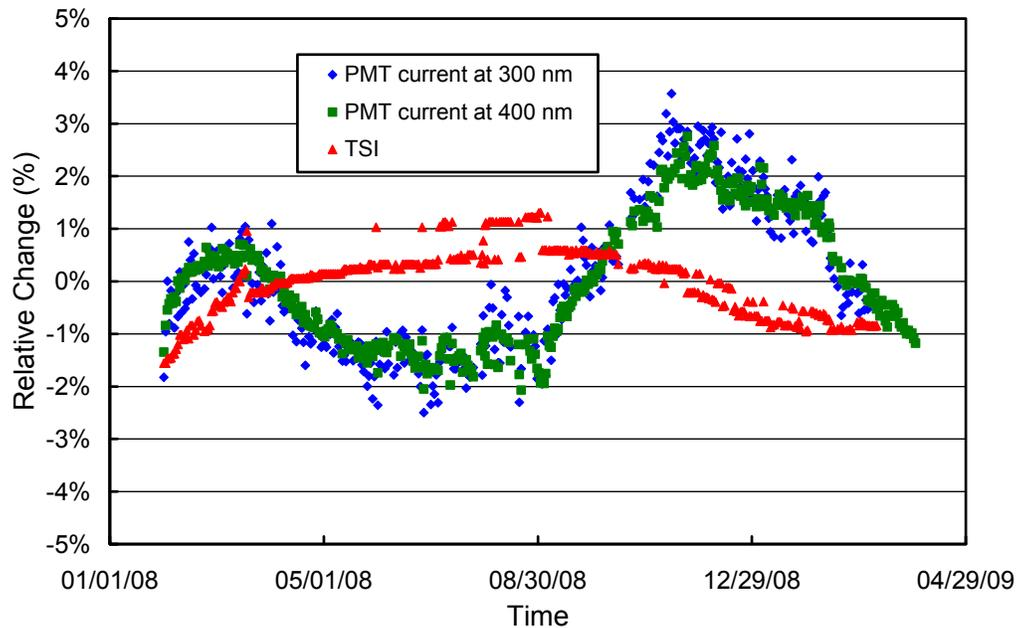
**Figure 5.1.3.** Time-series of PMT current at 300 and 400 nm, and TSI signal derived from measurements of the internal irradiance reference lamp during the McMurdo 2007/08 season. Data are normalized to the average value of the whole season.
