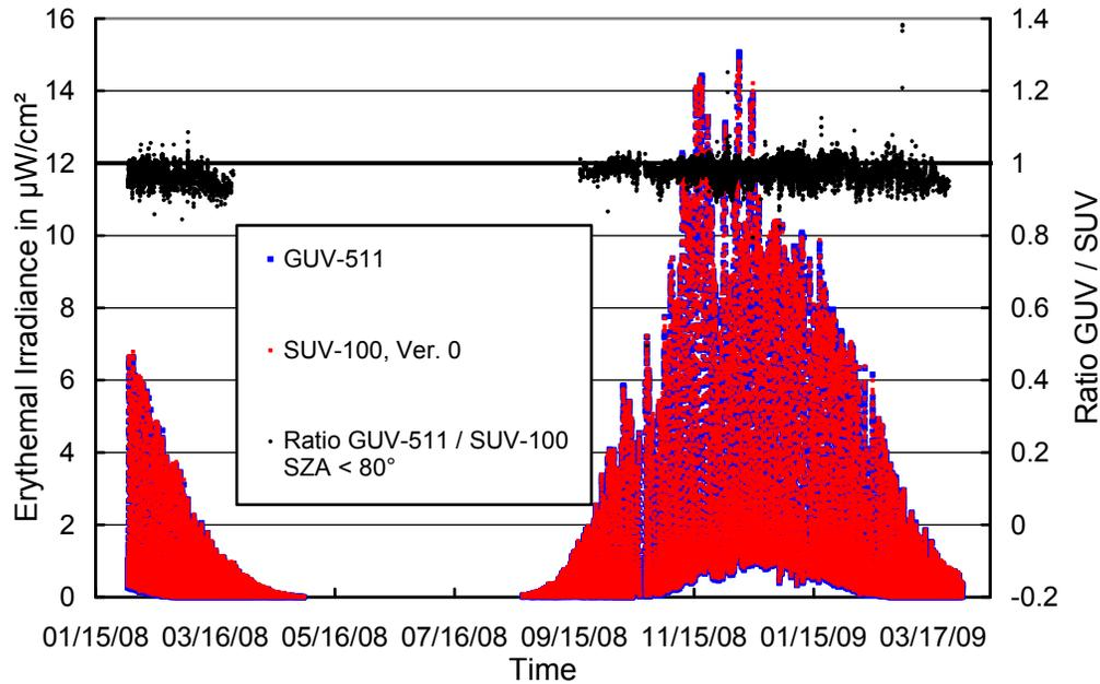
**Figure 5.1.9.** Comparison of erythemal irradiance measured by the SUV-100 spectroradiometer and the GUV-511 radiometer. All data are based on “Version 0” (cosine-error uncorrected) data.
