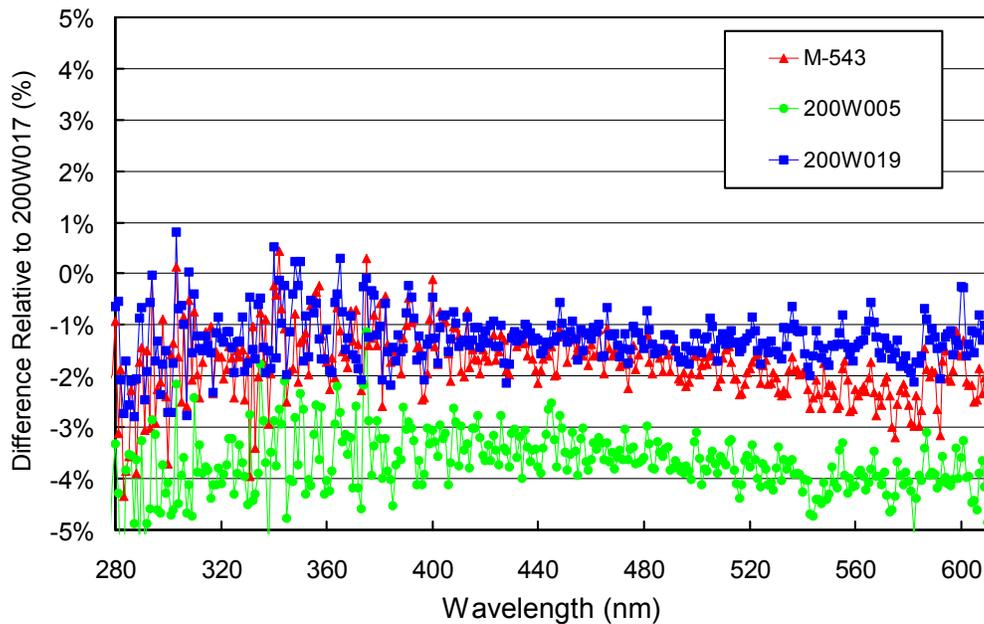
**Figure 5.1.2.** Comparison of McMurdo lamps M-543, 200W005, and 200W019 with the BSI traveling standard 200W017 on 2/11/09.
