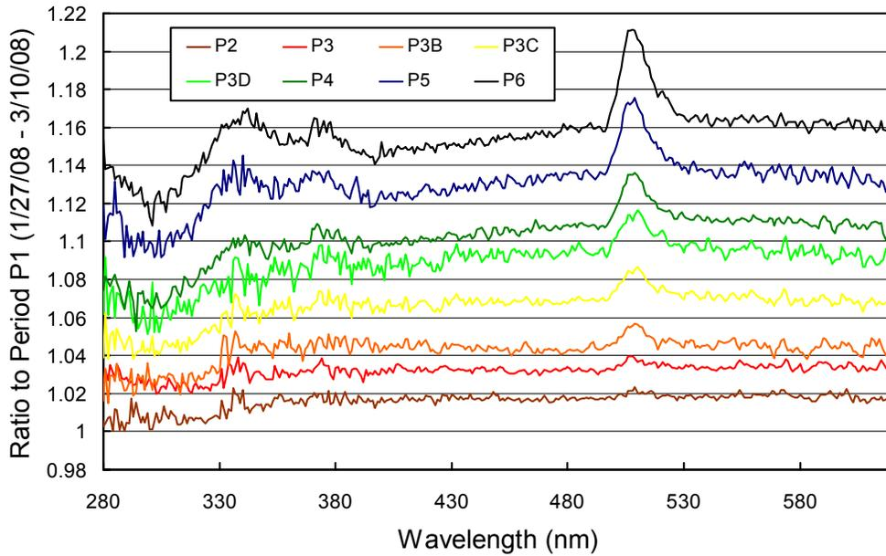
**Figure 5.1.4** Ratios of irradiance assigned to the internal reference lamp during periods P2 – P6, relative to Period P1.
