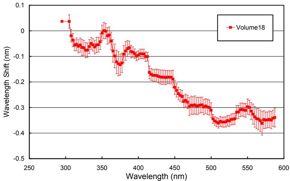
**Figure 5.1.7.** Monochromator non-linearity correction function. Error bars indicate the  $1\sigma$ -variation.
