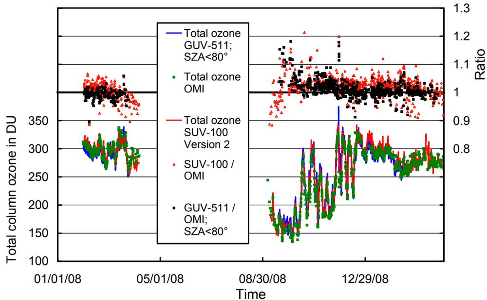
**Figure 5.1.10.** Comparison of total column ozone measurements from GUV-511, SUV-100 (Version 2 data), and OMI (v8.5, Collection 3). GUV-511 and SUV-100 measurements are plotted in 15 minute intervals. For calculating the ratio of both data sets, only GUV-511 measurements concurrent with OMI overpass data were evaluated. OMI measurements from 2009 are affected by an obstruction in the instruments field-of-view and have been removed from the dataset plotted.
