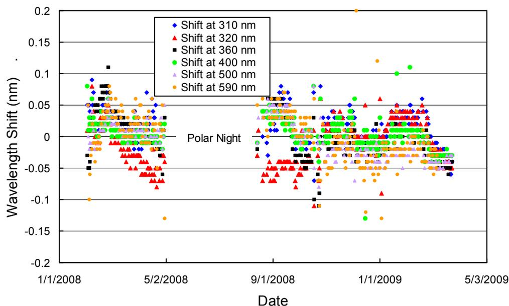
**Figure 5.1.8.** Check of the wavelength accuracy of final data at four wavelengths by means of Fraunhofer-line correlation. The noontime measurement has been evaluated for each day of the season. No correlation data is available during Polar Night.
