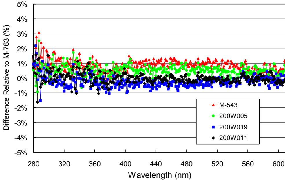
**Figure 5.1.1.** Comparison of McMurdo lamps M-543, 200W005, 200W011, and 200W019 with the BSI traveling standard M-763 on 1/29/08. Lamp M-763 had been calibrated in June 2007 against four 1000-Watt FEL standards provided by CUCF and corrected for the misalignment in its holder.
