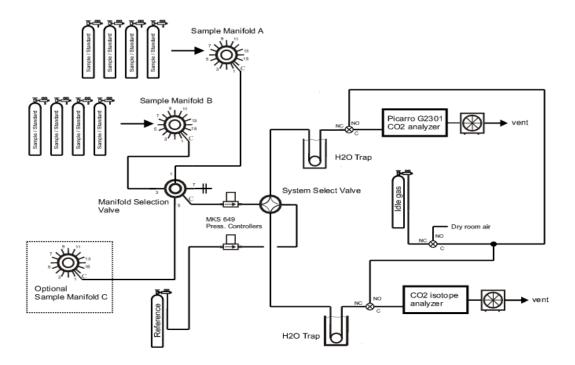
Figure 1: Plumbing diagram of combined CO<sub>2</sub> and CH<sub>4</sub> calibration system.
