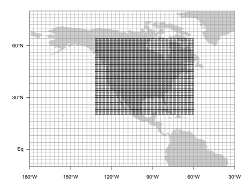
Figure 10: Nested grids used in CarbonTracker over North America. TM5 is a global model, but it employs nested grids to provide higher resolution over regions of interest. This figure shows the  $1^{\circ} \times 1^{\circ}$  nested regional grid over North America and a portion of the global  $3^{\circ}$  longitude  $\times$   $2^{\circ}$  latitude grid.
