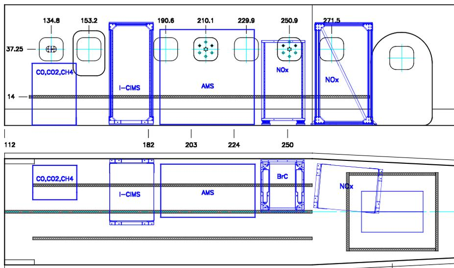
**Figure 5:** The potential payload for the NOAA Twin Otter for FIREX-CHEM: (1) CO, CO<sub>2</sub>, CH<sub>4</sub>, (2) O<sub>2</sub>, NO, NO<sub>2</sub>; (3) I-CIMS; (4) HR-AMS; (5) BrC-PILS.
