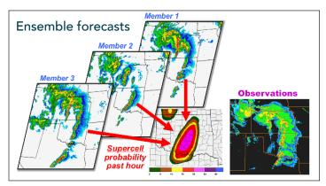
An example of how a range of solutions can converge on the most likely hazardous weather situation.
