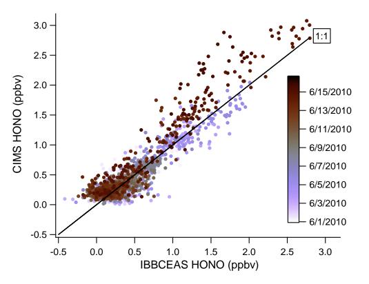
Removing the three vertical gradient days at the end of the campaign brings the in situ instruments into agreement, within 10%. • Good agreement between two in situ instruments.
