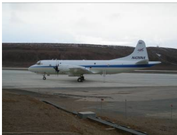
Wallops Flight Facility P-3B Flies from the surface to 20,000 ft 9 research instruments on board
