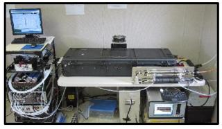
CRDS instrument to measure NO, NO<sub>2</sub>, NO<sub>y</sub>, and O<sub>3</sub>
