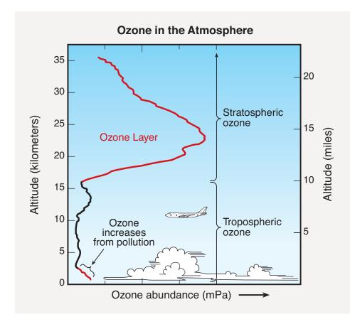
Figure Q1-2. Ozone in the atmosphere. Ozone is present throughout the troposphere and stratosphere. This profile shows schematically how ozone changes with altitude in the tropics. Most ozone resides in the stratospheric "ozone layer." The vertical extent or thickness of this layer varies from region to region and with season over the globe (see Q4). Increases in ozone occur near the surface as a result of pollution from human activities.
