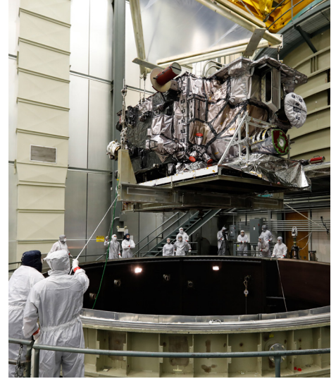
The GOES-17 satellite above the thermal vacuum chamber. Photo credit: Lockheed Martin.
