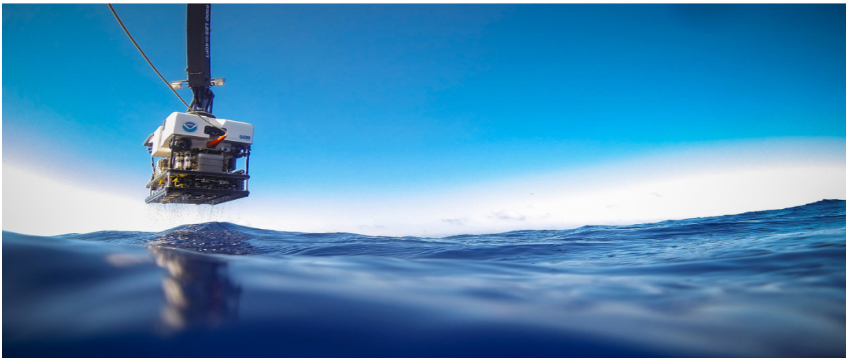
Remotely operated vehicle Deep Discoverer is recovered from a dive. Image courtesy of NOAA Okeanos Explorer Program, Gulf of Mexico 2014 Expedition.
