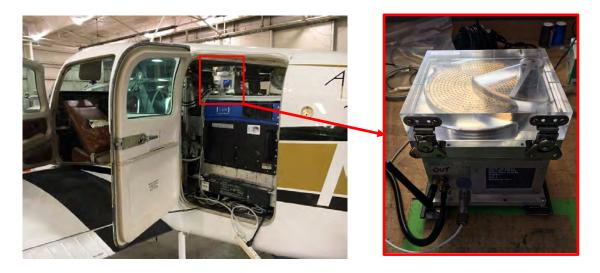
Weight: 10 lbs; Dimensions: H7"xW6.5"xD5.5" Input Voltage = 12-20VDC Power Supply Current Requirement = 1.5A Peak Current Draw = 1A Steady State Current Draw: 250mA
