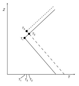
**Figure 5-20.** Simplified sketch of the sensitivity of the tropopause temperature and height with regard to changes of temperature in the stratosphere and troposphere. Solid lines: reference profile with cold point  $T_1$ . Long-dashed line with solid line: perturbed profile reflecting tropospheric warming with cold point  $T_2$ . Long-dashed line with short-dashed line: perturbed profile reflecting tropospheric warming and stratospheric cooling with cold point  $T_3$ . After Shepherd, 2002.
