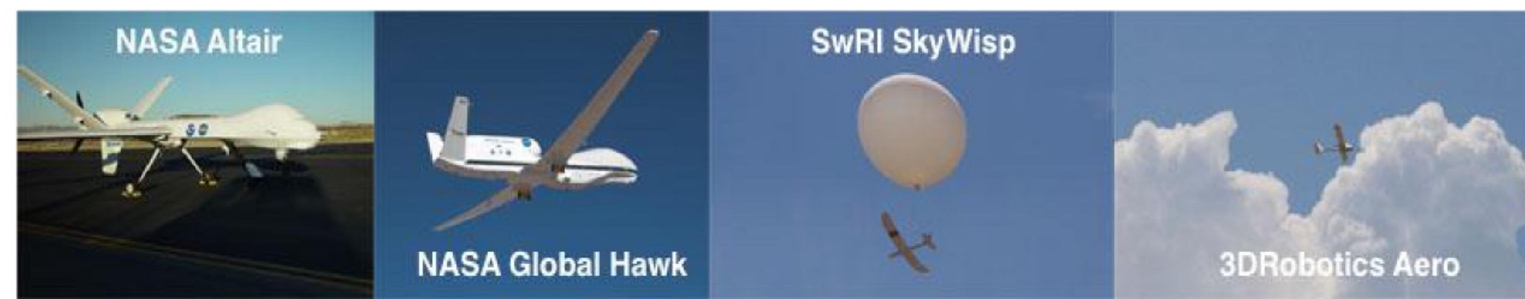
Figure 1 Collage of UAS platforms used left to right, including NASA Altair during NOAA 2005 Demo, NASA Global Hawk during ATTREX in 2014, SkyWisp (SwRI), and Aero (3DRobotics).
