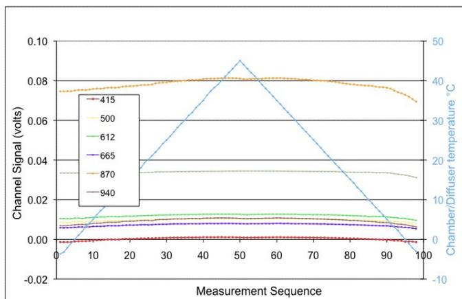
**Figure 1.** MFRSR channel voltage (left y-axis) output time series for a constant light source as the air temperature changes from -5°C to 45°C and back (light blue ramps, right y-axis).
