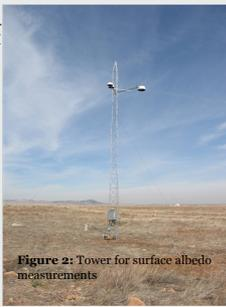
Figure 2: Tower for surface albedo measurements
