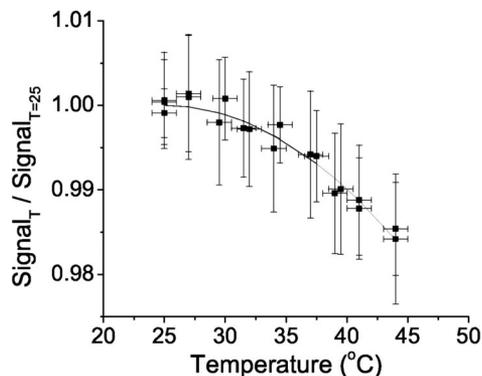
Fig. 1. Ratio of signals measured at different temperatures of the RIVM1 diffuser with reference to the lamp signal measured at  $T_{\text{dif}} = 25^{\circ}\text{C}$ .
