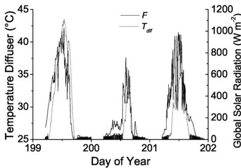
Fig. 3. Solar global radiation  $F$  and temperature of the diffuser  $T_{\text{dif}}$  for days 199–201 in 2004.
