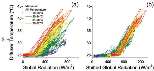
Fig. 4. (a) Weighted and (b) shifted weighted solar irradiances versus the diffuser temperature. The data are shown for several  $T_{\max}$  bins.
