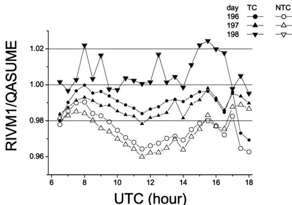
Fig. 6. Comparison of RIVM1 and QASUME with correction (TC) and without correction (NTC) of temperature dependence for days 196-198 in 2003.
