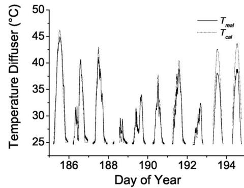
Fig. 5. Measured and retrieved diffuser temperatures for the period from 4 to 14 July 2006.
