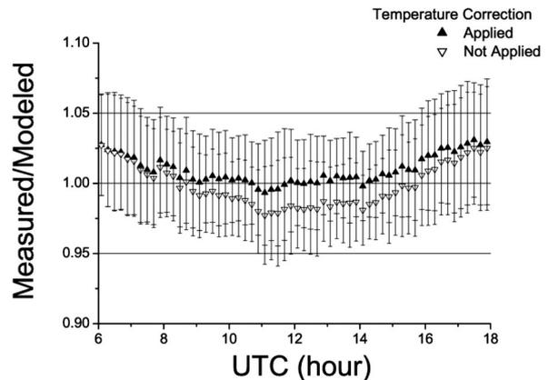
Fig. 7. Comparison of measured and modeled erythemal doses for clear sky days. Open triangles: temperature correction not applied; filled triangles, correction applied.
