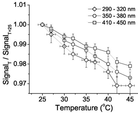
Fig. 2. Ratio of signals measured at different temperatures of the RIVM2 diffuser with reference to the lamp signal measured at  $T_{\text{dif}} = 25$  °C. The vertical error bars indicate the standard deviations of the wavelength averaging.
