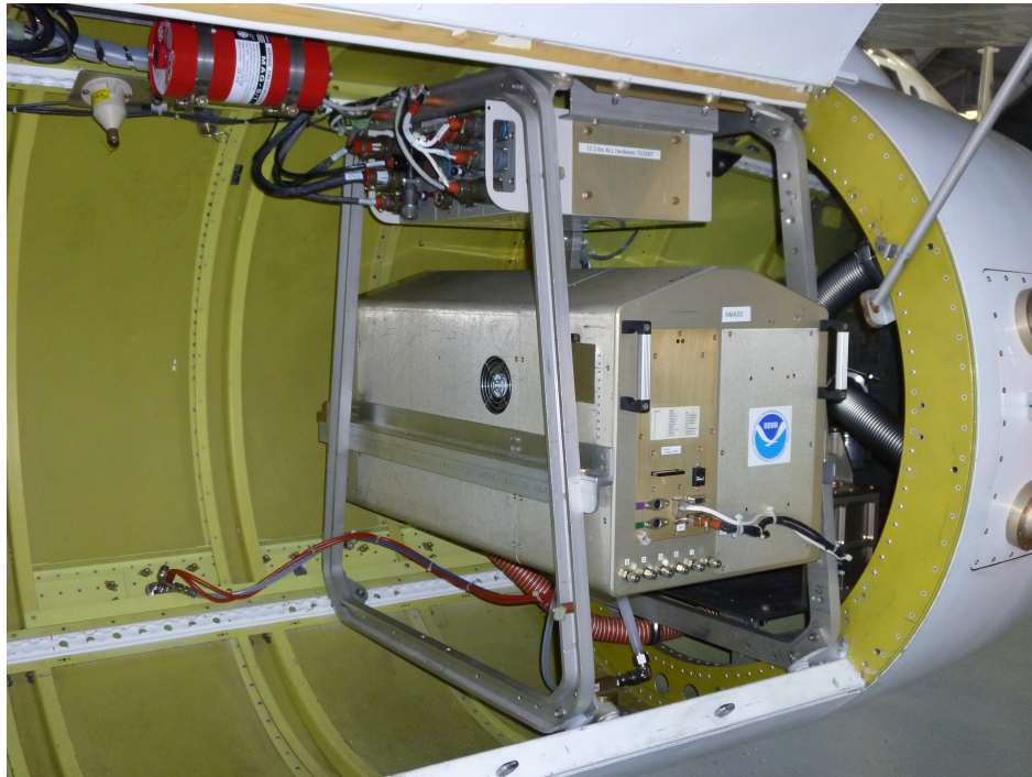
NMASS instrument in underwing pod of NOAA WP-3D aircraft.
